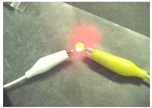
Fig.5: Glowing LED by voltage generation using a set up of MFC
