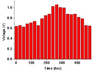
Fig.4: Voltage generation by MFC using Sewage wastewater with various electrodes when connected in parallel
