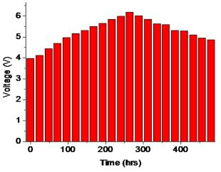
Fig.3: Voltage generation by MFC using Sewage wastewater with Pencil lead when connected in series
